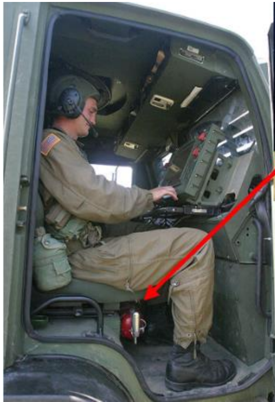
2.00" diameter Duocel® Aluminum Foam energy absorbers utilized in the FMTV increased crew protection cab seat mounts
